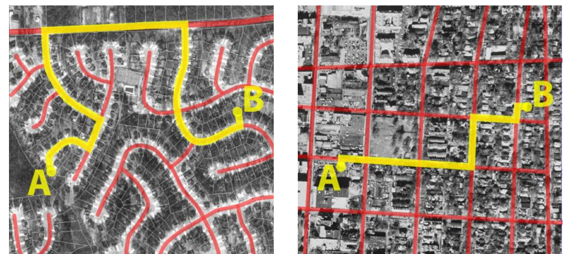
Good street connectivity is necessary for potential passengers to efficiently walk to transit stops.
